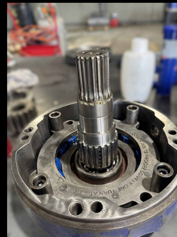
10SC Wet Brake during assembly
