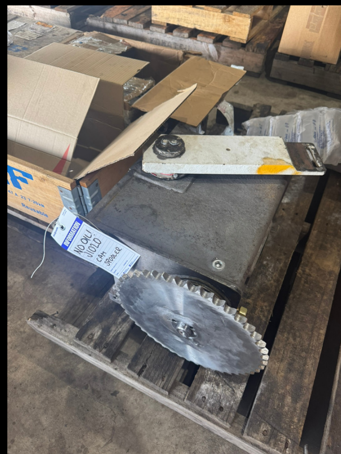
10SC Cam Spooler Overhaul
