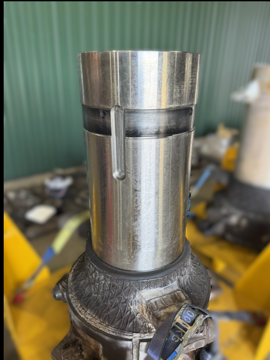
Cutter drum laserclad repair
