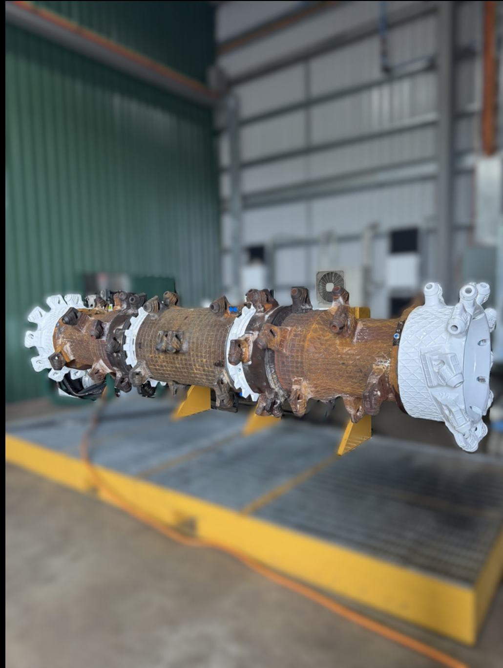
12CM Extendable Cutterhead Overhaul
